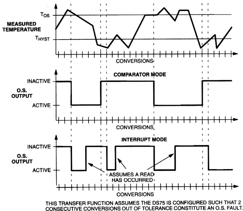
Regardless of the mode chosen, the O.S. output is open-drain and the active state is set in the configuration register. The power-up default is active low. Refer to the “OPERATION–Programming” section for instructions in adjusting the thermostat setpoints, thermostat mode, and O.S. active state.
