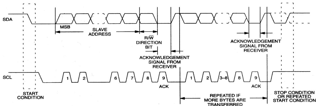
Figure 5 details how data transfer is accomplished on the two-wire bus. Depending upon the state of the R/W bit, two types of data transfer are possible:
